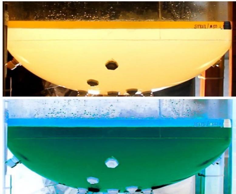
Figure 4: Separation between the phase's water and oil, a) original; b) contrasted
