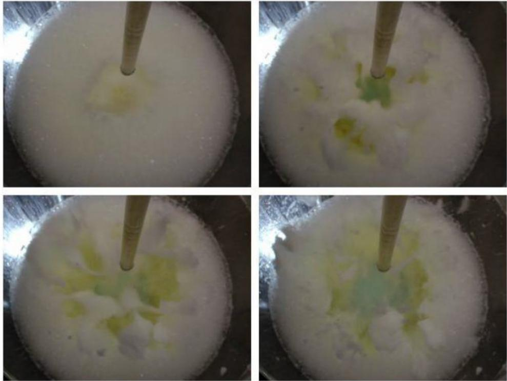
Figure 11: Initial air jet impact in the bath.
